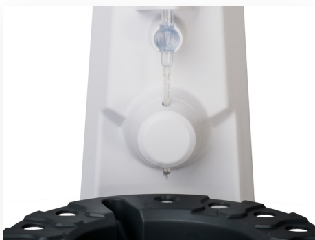
Figure 7: The nozzle tip centred over the flush hole. Note that for the side of the carousel that holds 2 mL tubes, the flush hole will be on the right of the central well channel. For the other side of the carousel that holds 5 mL tubes, the flush hole is on the left of the central well channel.
